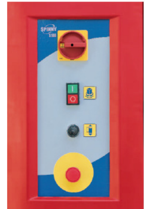
Spinny S100 Control panel
