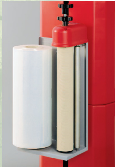
Adjustment of film tension through mechanical brake
